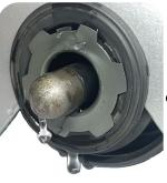
A few drops of water within the caliper can cause corrosion and lead to caliper failure.
