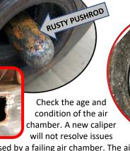
caused by a failing air chamber. The air chamber's internal seals can fail, thus causing contaminates to enter the air chamber and caliper. If the air chamber's condition cannot be verified or is questionable, replace the air chamber when the ADB caliper is replaced.
