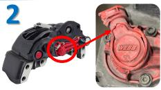
Examine the caliper's chain cover for cracks or damage and replace as required. Replace the caliper if water has caused rusting on the internal components.
