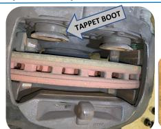
Inspect tappet boots for tears or heat damage that could allow moisture to enter the brake caliper and replace as required.
