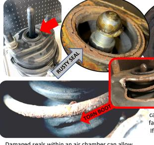
Damaged seals within an air chamber can allow moisture to enter the brake caliper.
